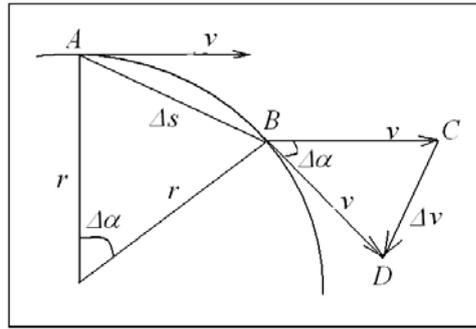
$$v = \frac{\Delta s}{\Delta t} = \frac{2r \sin \frac{\Delta \alpha}{2}}{\Delta t}; \quad \Delta t \rightarrow 0, \Delta \alpha \rightarrow 0, \sin \frac{\Delta \alpha}{2} = \frac{\Delta \alpha}{2}$$
